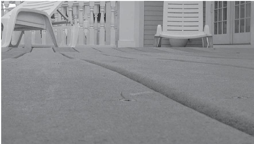
**Figure 12.4** Distortions of WPC deck boards due to water absorption.
